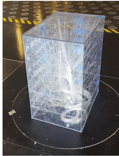
Figure 2 – The 24-story building model (1:120 scale) placed in the wind tunnel for testing at the University of Florida.
